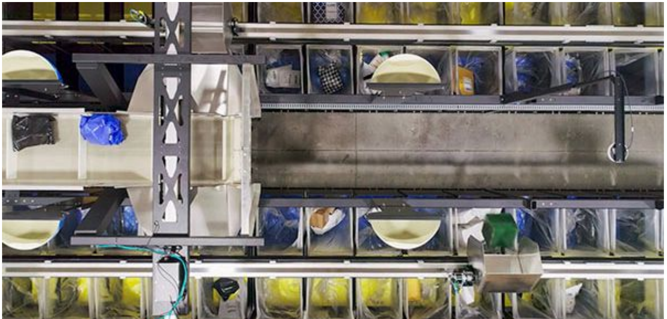
Automated systems, such as Berkshire Grey's Robotic Process Sortation and Identification (RPSi), can take on tedious returns sortation tasks, expediting reverse logistics workflows. Source: Berkshire Grey
