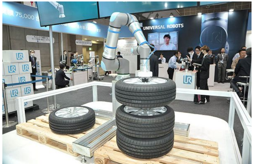
Universal Robots new UR30 cobot has a payload capacity of 30 kg. Source: Universal Robots
