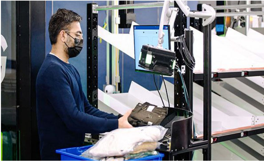
Automated systems, such as Berkshire Grey's Robotic Shuttle Putwall, can handle returns sortation tasks, allowing employees to address fraudulent returns. Source: Berkshire Grey
