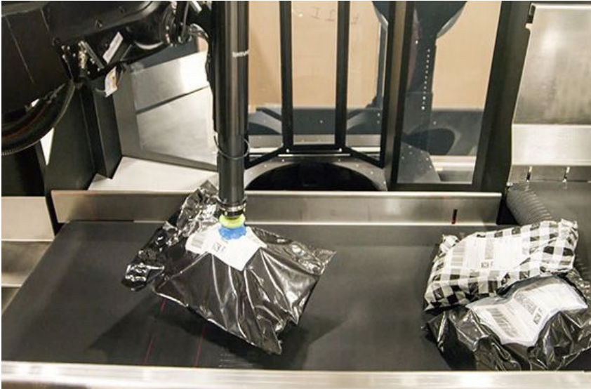
Berkshire Grey's Robotic Process Sortation and Identification (RPSi) can pick items off conveyor belts, release them through a barcode scan tunnel, then sort the product into a cubby or bin. Source: Berkshire Grey
