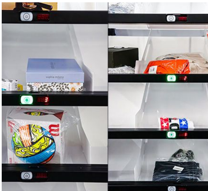
Berkshire Grey's Robotic Shuttle Putwall (RSPW) can sort small boxes and items in poly bags to expedite reverse logistics workflows. Source: Berkshire Grey
