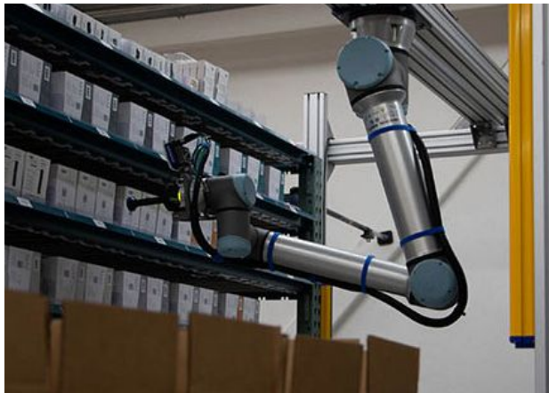
DCL Logistics chose the UR10e for its pick-and-pack process, reducing its labor costs by 50%. Source: Universal Robots
