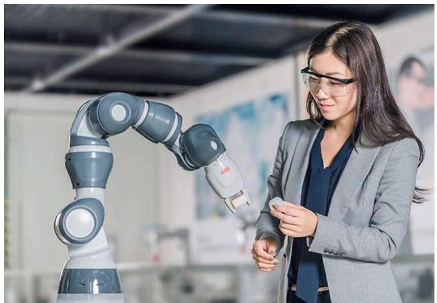
Cobots such as the single-arm YuMi are designed to be easy to program. Source: ABB
