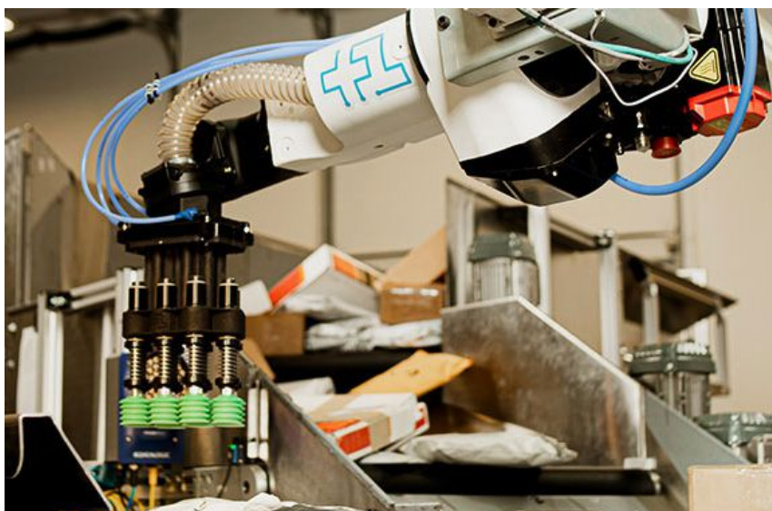
Through a combination of supervised autonomy and adaptable AI purpose-built for parcel picking, Plus One enables robot arms to handle variable package types. Source: Plus One Robotics
