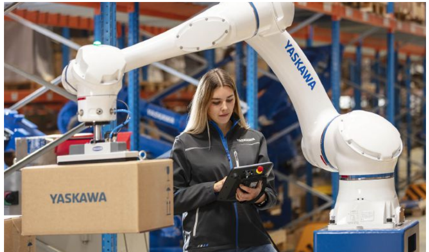
Yaskawa Motoman's HC series, or "Human Collaborative" cobot arms, include safety features and easy-to-use programming tools that enable flexible deployment options. Source: Yaskawa Motoman
