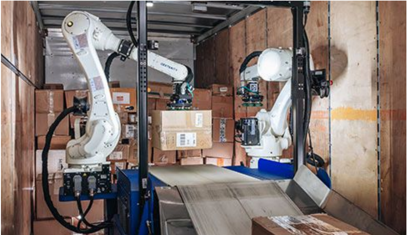
The Dexterity DexR is an AI-enabled robot with two robot arms that precisely build walls in a truck. Source: Dexterity
