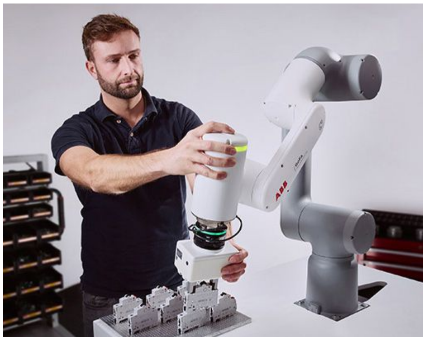
Ease-of-use technologies, such as lead-through programming, graphical user interfaces, and offline programming, are clearing the way for broader robotics adoption. Source: ABB
