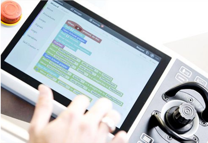
Software like the ABB Wizard Easy Programming shown here allows small and midsize manufacturers to bring robots online without specialist skills or knowledge of RAPID code, facilitating the use of robotic automation in production lines. Source: ABB
