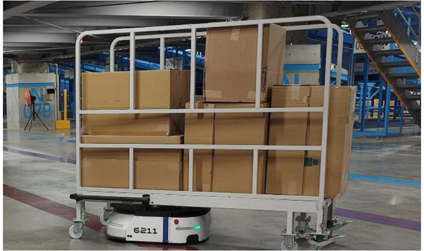
The LexxPlus Sagawa can carry boxes on a cart above the AMR. Source: LessPluss
