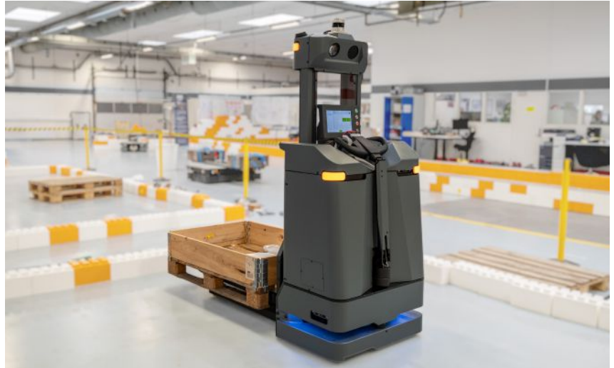
Through NVIDIA Jetson AGX Orin, the MiR1200 autonomous pallet jack combines data from four RGBD cameras and 3D LiDAR to detect obstacles and navigate autonomously. Source: MiR
