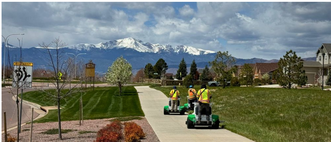
Landscapers drive their fleet of Scythe Robotics M.52 mowers out to a property. Once the robots are in their respective mow zones, the operators simply press start to begin autonomous Scythe mode. Source: Scythe Robotics
