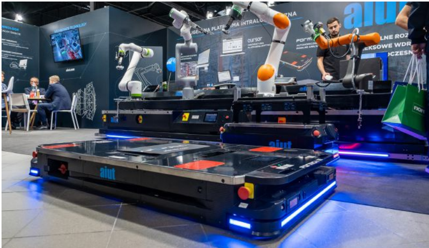
AFORMIC's low-profile F12 AMR is designed for automating transportation logistics operations within manufacturing plants. Source: AFORMIC
