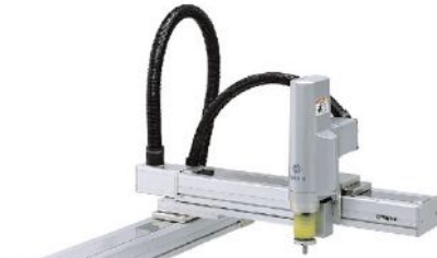
Yamaha makes Cartesian robots for clean room applications. Source: Yamaha
