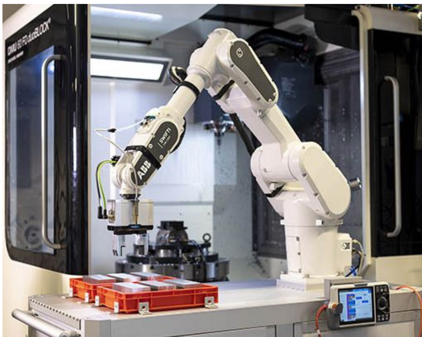
The SWIFTI CRB 1300 cobot is intended to be fast and accurate enough for a variety of industrial applications. Source: ABB
