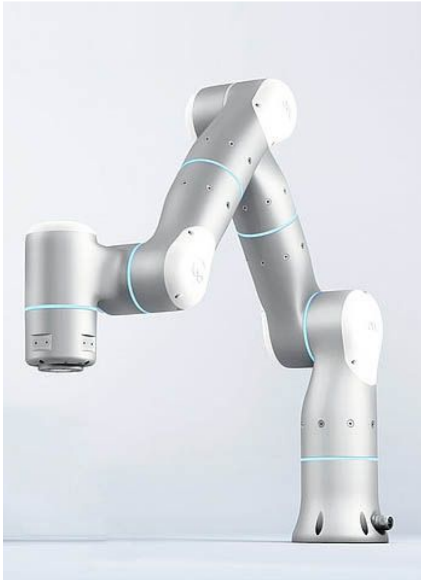
The Rizon 10 has seven degrees of freedom. Source: Flexiv
