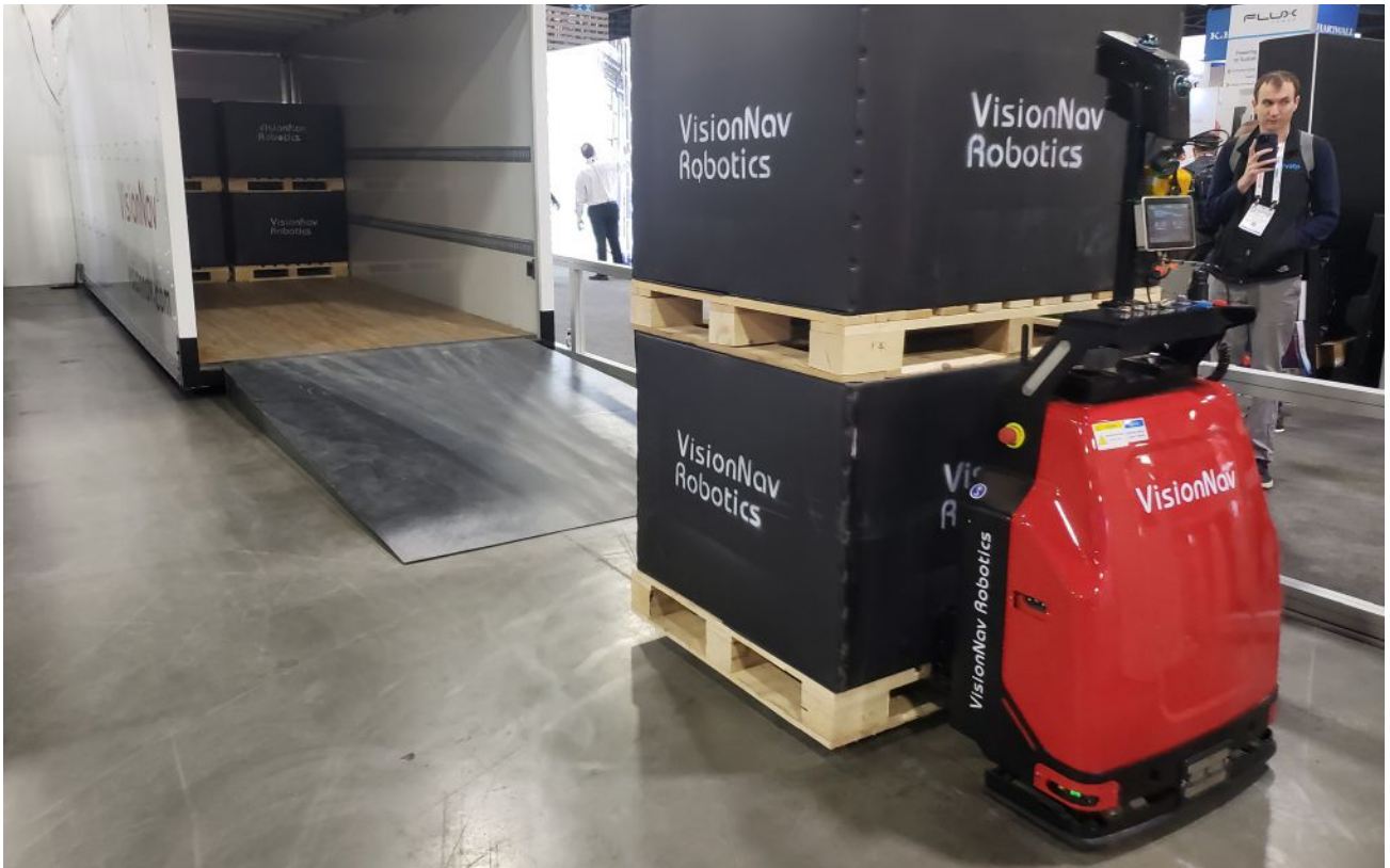
VisionNav's VNST20 PRO AGV has been designed specifically for automated loading and unloading of trailer trucks, incorporating 3D lidar and SLAM machine vision. Source: Donald Halsing, Peerless Media
