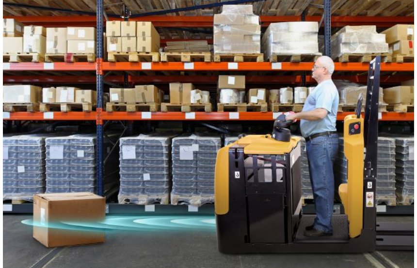
Thanks to machine vision and lidar, Yale lift trucks are able to identify potential hazards. Source: Yale Lift Truck Technologies
