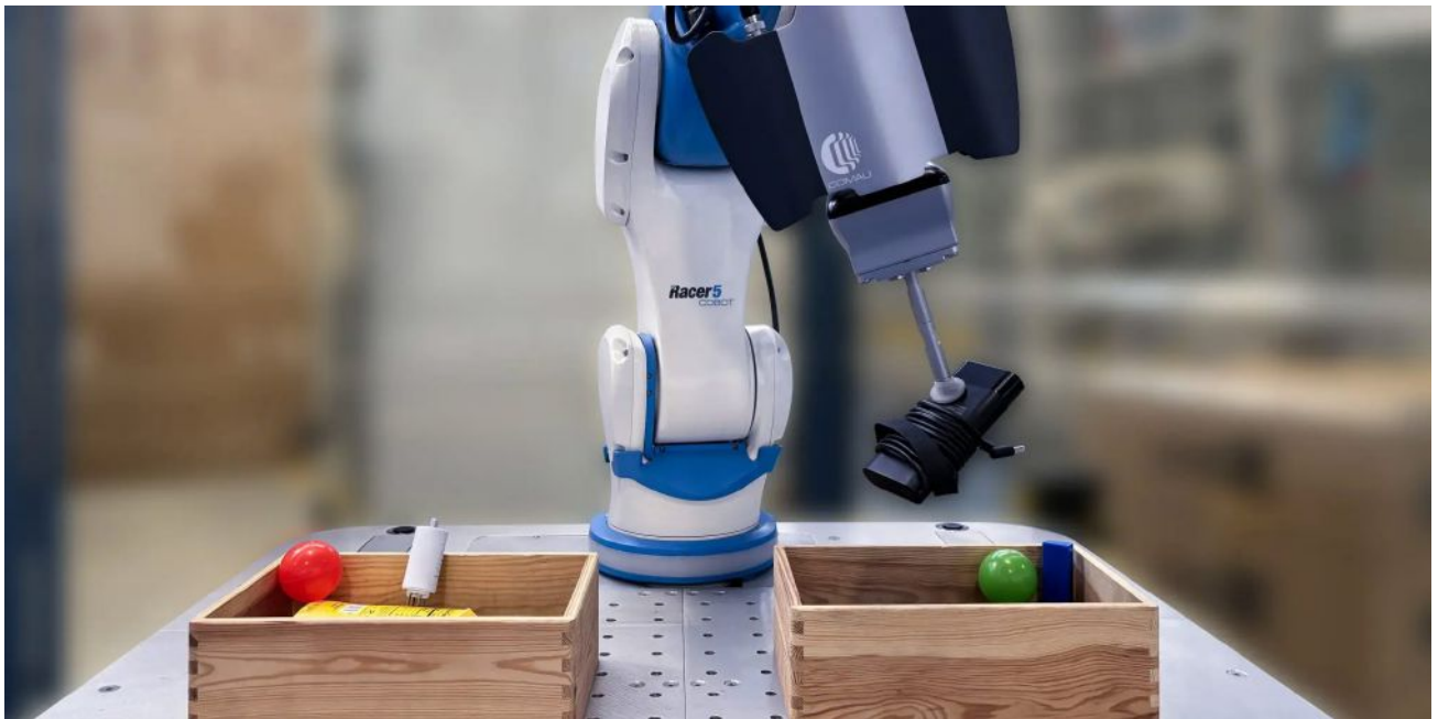
Comau's new MI.RA OnePicker AI-backed vision system can pick miscellaneous objects from bins without prior information. Source: Comau
