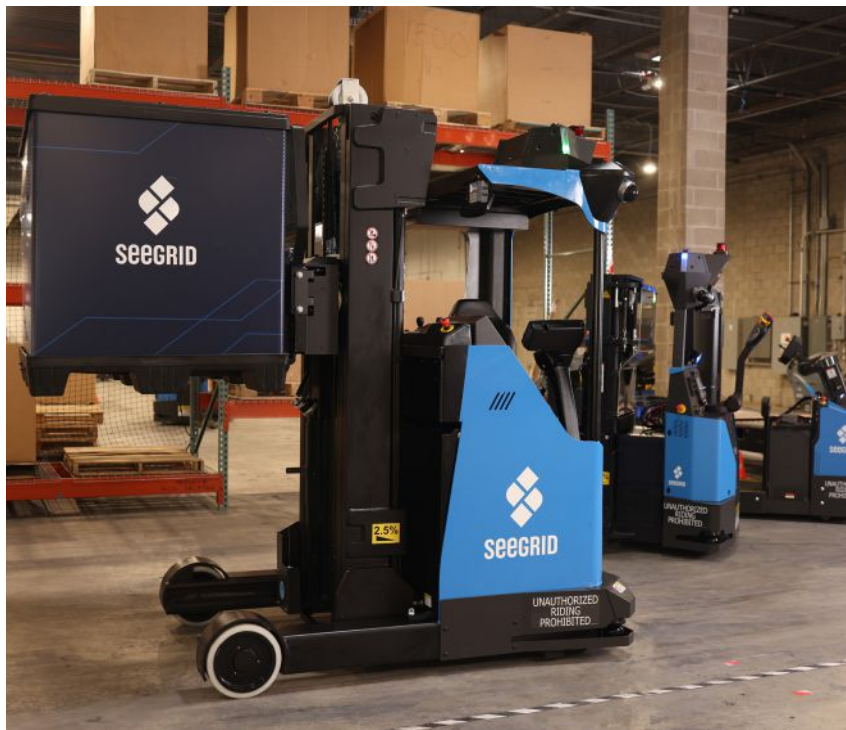
Seegrid's autonomous lift trucks are capable of precisely picking, moving, and placing pallets - a task which depends on industry-ready machine vision hardware and software. Source: Seegrid
