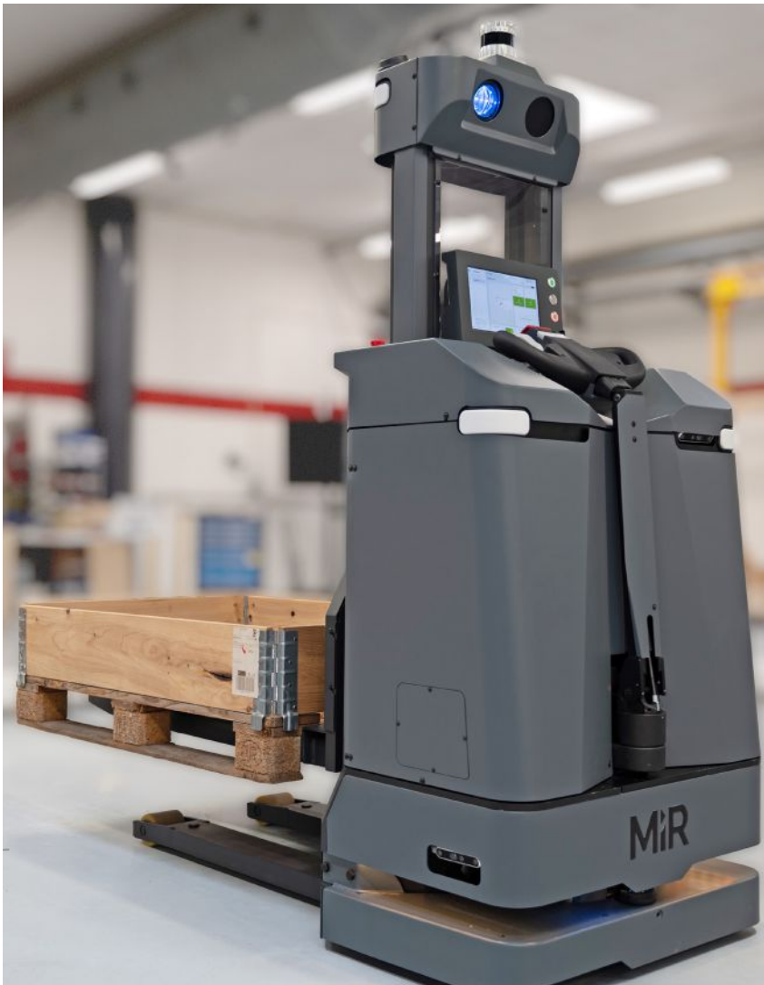
Through NVIDIA Jetson AGX Orin, the MiR1200 autonomous pallet jack combines data from four RGBD cameras and 3D LiDAR to detect obstacles and navigate autonomously. Source: Mobile Industrial Robots (MiR)
