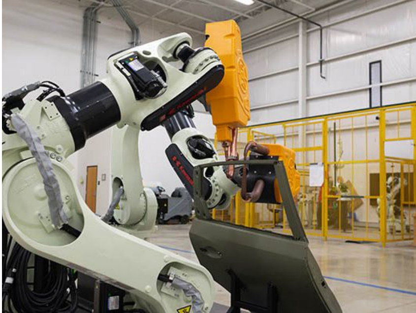
Kawasaki will demonstrate a BX100N robot welding a car door using the RapidPlan software. Source: Realtime Robotics
