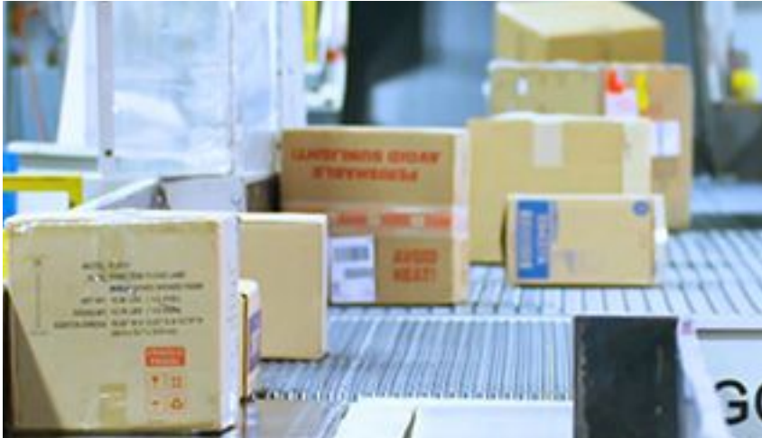
Activated Roller Belt (ARB) Singulator for large parcels. Source: MHS
