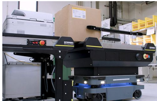
A MiR AMR demonstrates the transfer of a box to a conventional conveyor. Source: Mobile Industrial Robots
