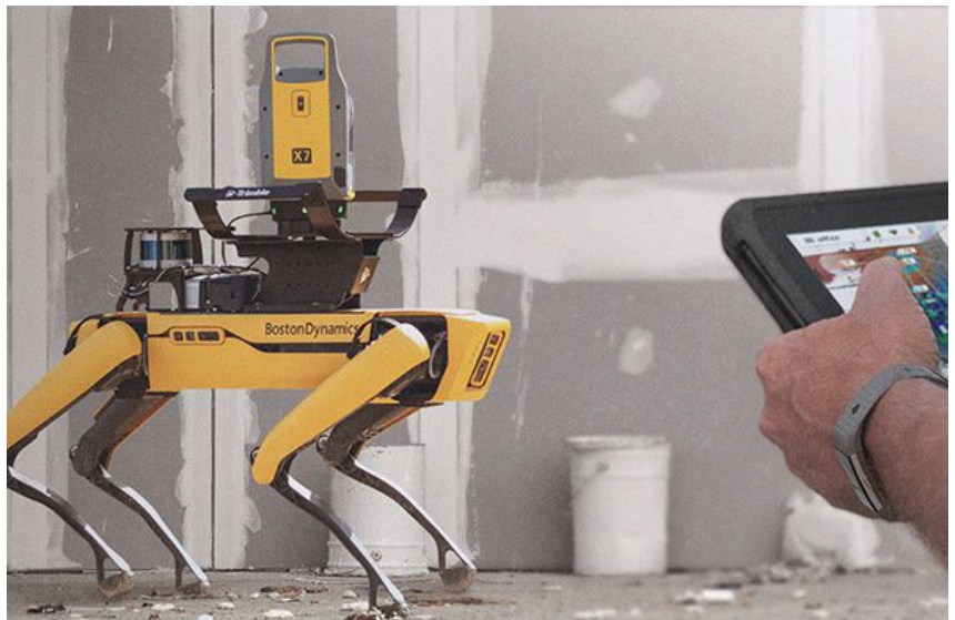
Trimble's X7 3D laser scanner and FieldLink software are integrated with Boston Dynamics Spot quadruped for autonomy on construction sites. Source: Trimble
