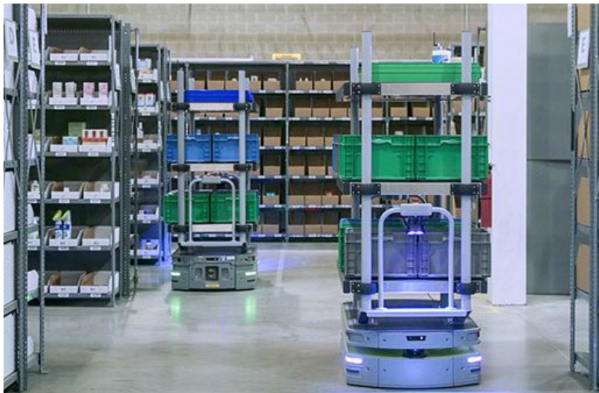
The Meet Me person-to-goods system includes Lumabots (above) and the Pyxis software. Source: Onward Robotics
