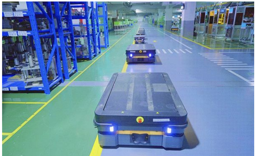
AMRs automate the movement of pallets and assembly parts without extra infrastructure. Source: Mobile Industrial Robots
