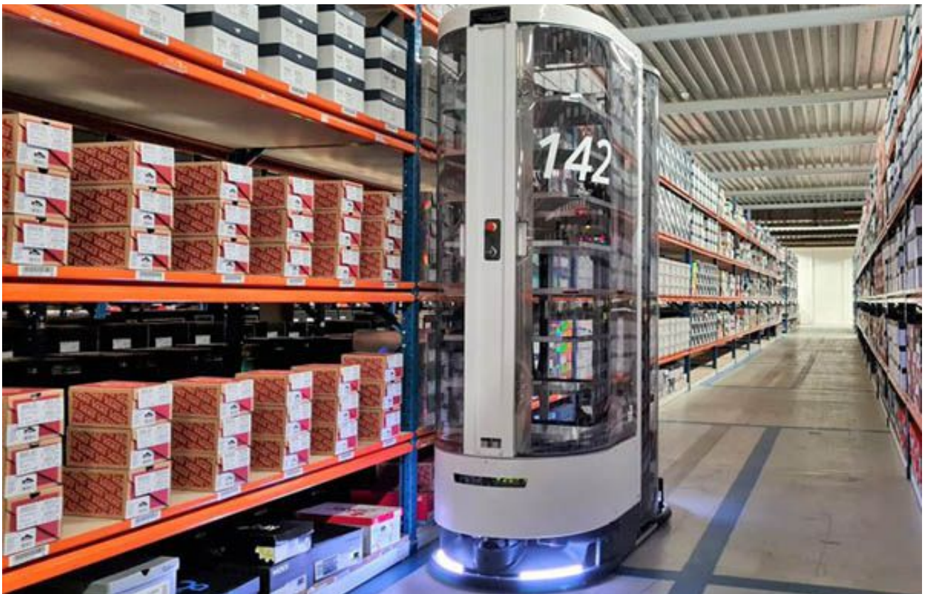
The TORU robot has a payload capacity of 40 kg (88 lb.). Source: Magazino
