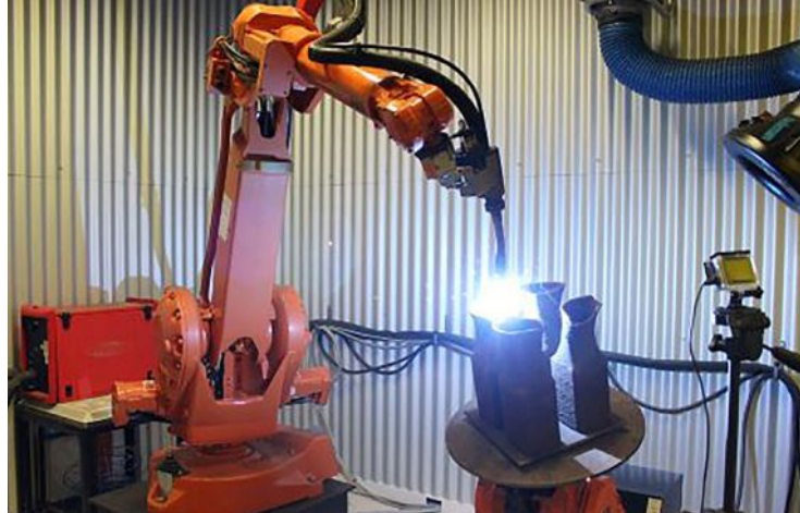
TiDA Ltd.'s robotic welding 3D-printing system in action, using WAAM technology. Source: The University of Waikato
